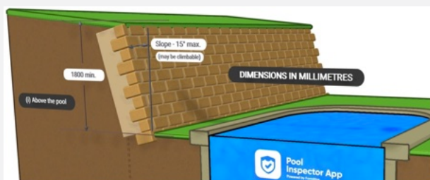
Retaining wall above the pool
