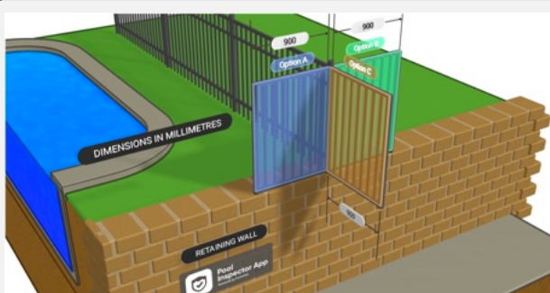
Where a barrier meets a retaining wall
